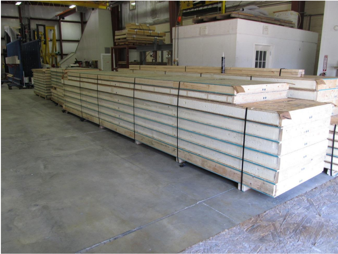
Figure 3: Net Zero SIPS LLC, Structural Insulated Panels
